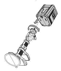
By means of the suction cup you can affix the mount to smooth surfaces such as tiles or glass.
