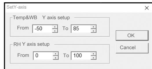
1. Enter the desired temperature scale values (on the left of the graph) and the relative humidity scale values (on the right of the graph).
