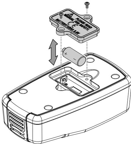
3. Close the battery compartment (5) and secure it by remounting both screws.
